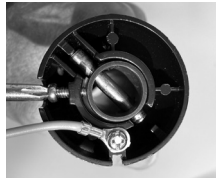
remove half-ball and stopper pin
