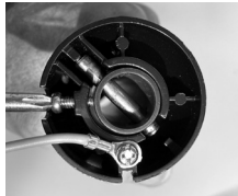
remove half-ball and stopper pin
