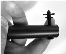
remove stopper pin assembly
