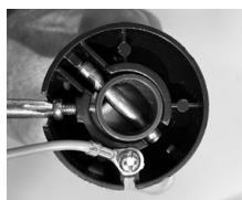
remove half-ball and stopper pin
