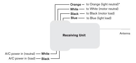
\* If fan does not have orange wire, cap orange wire from receiving unit.
