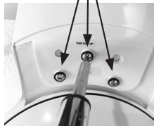
blade screws with rubber washers
