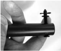
remove stopper pin, cotter pin and washer
