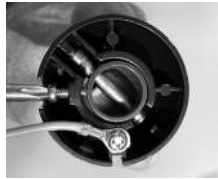
remove half-ball and stopper pin
