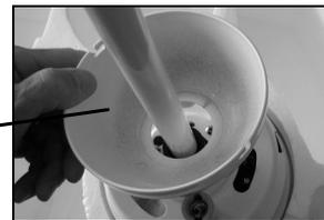
(9) Reinstall half ball from step (5) on end of down rod. Be sure that stopper pin is inserted through down rod and seated in half ball. Tighten set screw against down rod.
