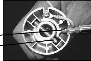
(6) Replace top cover from **step (3)**, ensuring "reverse" switch opening is properly located. Then remove the stopper screw and loosen the set screw on the fan collar. Set the stopper screw aside for **step (7)**.
