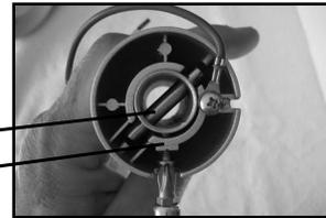
**(7)** Remove the stopper screw and loosen the set screw on the fan collar. Set the stopper screw aside for step **(8)**.
