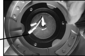
**(4)** If your fan does not have a light, position light lead wires against large washer and place lighting plate on flange so that wires key holes fit over two screws on flange. Be sure wires are clear of edges and completely contained in the center cavity. Rotate plate and reinstall third screws from step **(3)**. Tighten all three screws. If your fan does have a light, make quick connect wire leads and prior to attachment of light plate.
