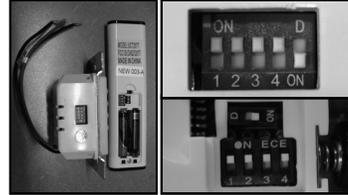
Locate the dip switches as pictured to right, and carefully select a new combination of "on" and "off" switches. Within 60 seconds of turning the AC power on, press and hold down the "fan off" button for five seconds. The receiver will then lock in the chosen frequency. Test operation to confirm transmitter and receiver are synced together. If using a handset and wall switch in combination (#005) the dip switches must match.
