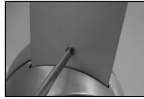
**(23)** Using the pan head screws labeled BLADE SCREWS in the hardware package, attach the inside edge of each blade to the rotor. Do not tighten screws all the way until both inside screws and the outside "CENTER" screw from step **(22)** has been partially started for each blade. Take care not to cross thread the screws.
