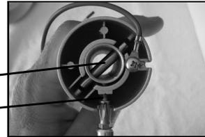
(13) Slightly loosen two screws where down rod is to be installed in step (14).
