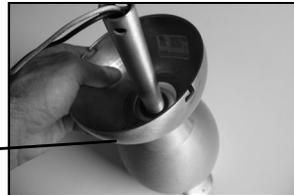
(17) Reinstall half ball from step (12) on end of down rod. Be sure that stopper pin is inserted through down rod and seated in half ball. Tighten set screw against down rod.
