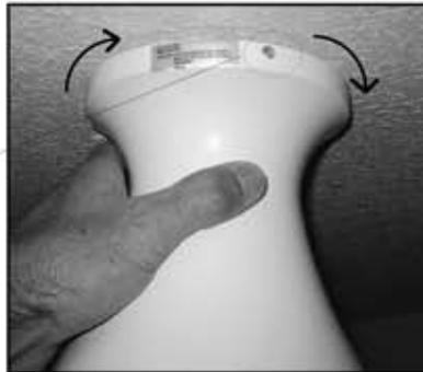
**(5)** Insert and firmly tighten three canopy screws. Hint- do not tighten down canopy screws until all three are partly screwed in.
