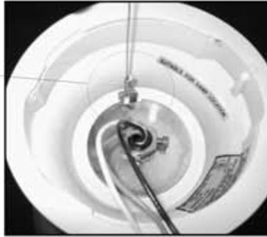
**(4)** Lift fan body and carefully align collar with ceiling plate. Tabs on ceiling plate should seat into channel on inside of fan collar. Rotate fan so that canopy screw holes on fan body align with canopy screw holes on ceiling plate.
