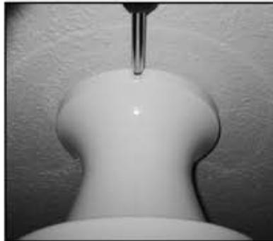
**(6)** Carefully insert the lamp into the socket and the two lamp holders. The brass pins on the lamp snap into the socket.
